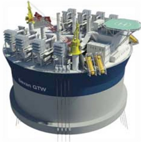
Figure 12.2 Ship/island for the processing of natural gas, including liquefaction facilities and loading onto natural gas tankers.
