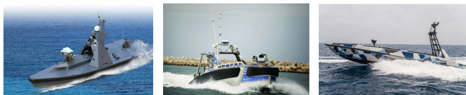
Figure 5: From left to right: The Protector developed by Raphael, 49 the Katana developed by Israel Aircraft Industries 50 and the Seagull system developed by Elbit 51
