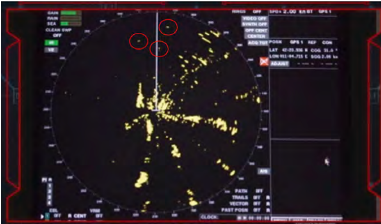
Figure 5: The actual RADAR display that shows the obstacles that were concealed from the navigation officer using manipulation
