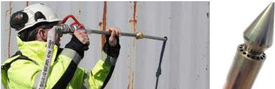
Figure 10: Water-Mist Lance, capable of penetrating the container's side
