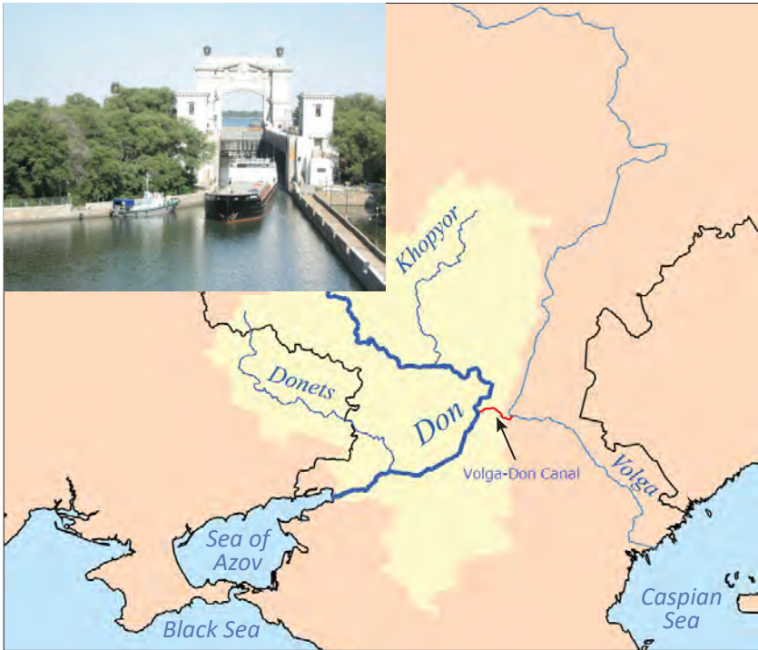
Figure 2: The shipping route connecting the Caspian Sea with the Sea of Azov and the Black Sea through the crossing of the Volga and Don rivers and the canal connecting them. In the picture is gate number 14 of the Volga-Don Canal
