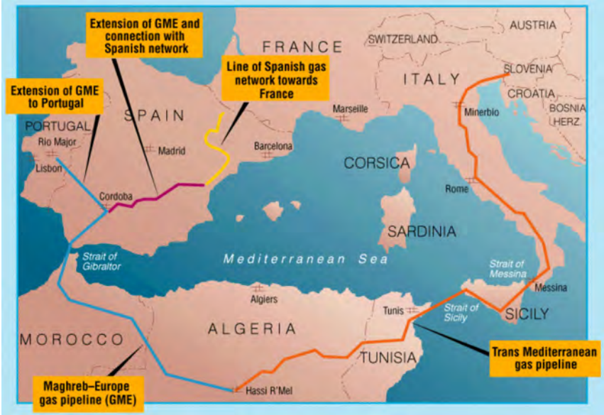
Figure 4: The gas pipelines from Algeria to Italy (in orange) and Spain (in blue), and the gas pipeline from Spain to France (in yellow) 25
