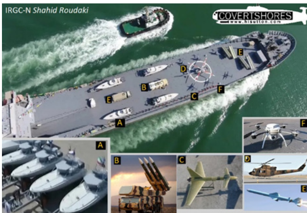
Figure 13: The Roudaki – top view with its various equipment and naval armaments. It carries an assortment of weapons on board (speed boats, sea-to-sea missiles, a helicopter, UAV's, a vehicle carrying anti-aircraft missiles)
