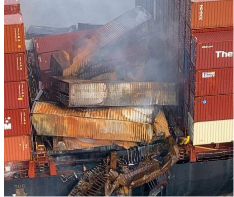
Figure 8: Damage and burn due to collapse of containers, ZIM Kingston, October 2021 10
