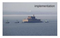
The platform is relative small in size  $-10 \times 30 \times 145$  meters with a draft of about 5 meters. According to its planners, its can withstand the local conditions.
