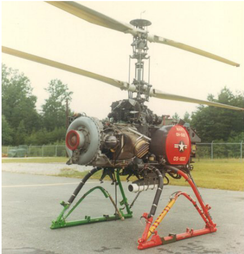
Figure 3: A SNOOPY helicopter equipped with a camera and a transmission device (Gyrodyne.com)
