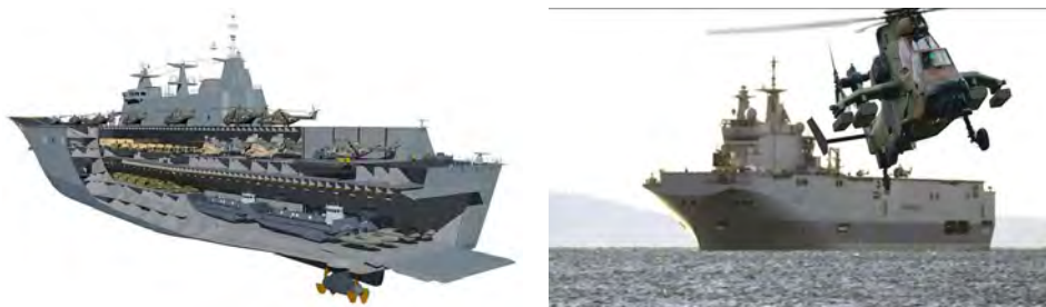
Figure 2: Left – A cross-section view of the vessel including the configuration for carrying landing craft, armored vehicles and helicopters. Right – Ka-52 attack helicopter takes off from the deck of a Mistral 28 ship.
