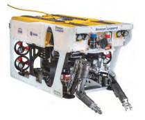
A work class Remotely-Operated-Vehicle (ROV), capable of operating to 3,000m depth, equipped with 11 powerful electric thrusters for outstanding maneuverability, a Schilling Orion 7P manipulator, cameras, survey sonars and a dedicated scientific skid allowing the installation and testing of additional sensors and the collection and storage of samples.
